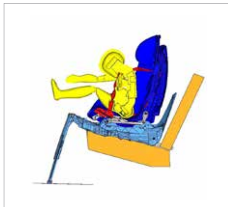
HyperWorks frontal impact simulation, simulation, forward and rearward facing positions.
