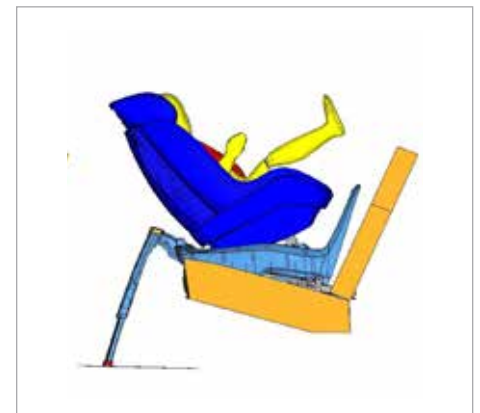
HyperWorks frontal impact simulation, simulation, forward and rearward facing positions.
